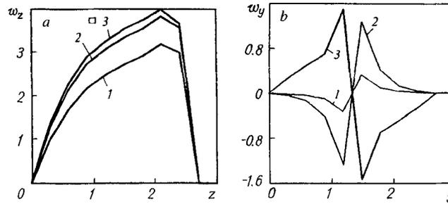
Fig. 3. Distributions of the projections of the velocities of the gas medium at different instants of time from the onset of combustion: a)  $w_z$ : calculation: 1) 10 sec; 2) 30 sec; 3) 60 sec; the points, experiment [11]; b)  $w_y$ : 1) 0.05 sec; 2) 1 sec; 3) 5 sec.  $w_z$ ,  $w_y$ , m/sec;  $z$ ,  $y$ , m.
