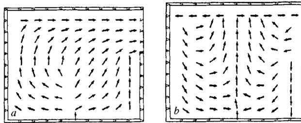
Fig. 4. Characteristic fields of the velocities of gas flow at different instants of time: a) 0.1 sec; b) 5 sec.
