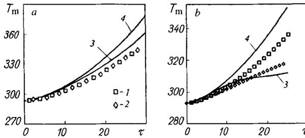
Fig. 1. Dependences of the mean-volume temperature on the time from the onset of combustion ( $\Pi = 0.01$  (a);  $0.28$  (b)): 1) analytical solution [2]; 2) integral model [2]; 3, 4) proposed model: 3) the opening is at the top; 4) the opening is at the bottom.  $T_m$ , K;  $\tau$ , sec.
