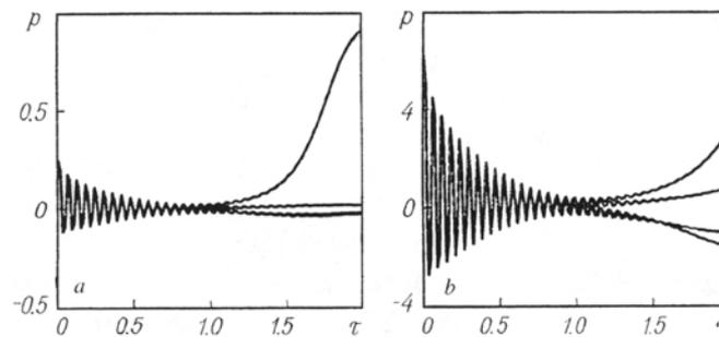
Fig. 6. Dependence of the pressure on time:  $F = 0.01$  (a);  $0.25$  (b).  $p$ , Pa.
